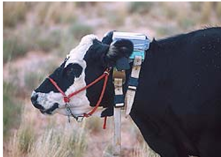
The prototype virtual fence device as a neck saddle.
