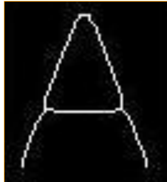
Skeleton after 6 applications of spur removal algorithm.
