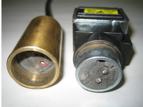
Figure 8 - Solenoid failed after HALT test
