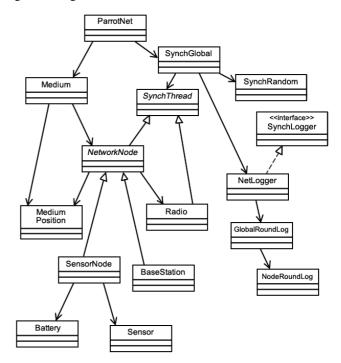
Figure 4. ParrotNet Class Diagram for Simulation
