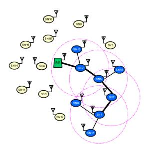
Figure 2. ParrotNet virtual path example: the delivery of data from sensor node SN1 to base station (BS).
