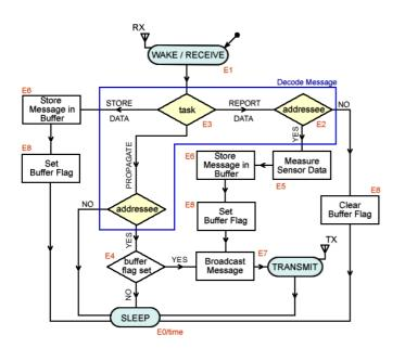
Figure 1. Sensor node functioning flow diagram.
