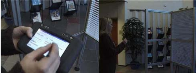
Figure 7. Shutter control solution based on 6LoWPAN communication.
