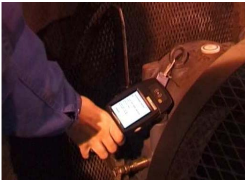
Figure 1. Identifying greasing task location with mobile RFID reader (UHF).
