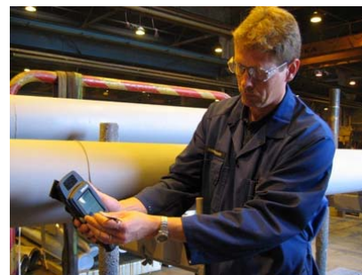
Figure 6. Identifying pipes in production line with Psion WAP G2 reader.
