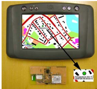
Figure 8. Requested geosensor information with Kitwrx 456 device.
