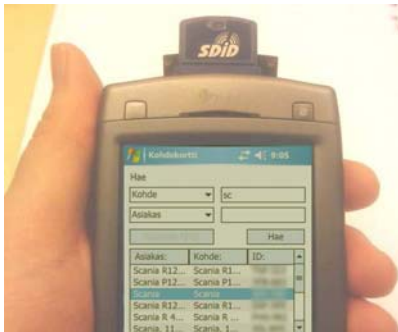
Figure 4. A mobile device with RFID adapter for maintaining vehicles.
