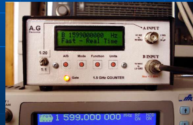
Photo of the implemented frequency counter during test measurement
