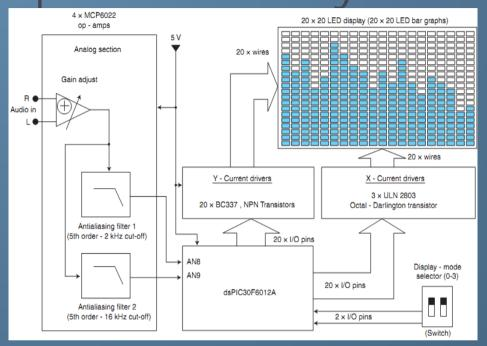
Current < 600 mA, because are not powered simultaneously, but are cycled using scanning technique.  In this figure we can see the complete design of the Digital Audio Spectrum Analyzer as a block diagram.
