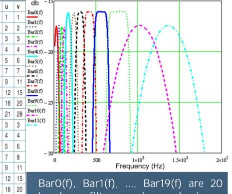
BarO(f), Bar1(f), ..., Bar19(f) are 20 bandpass filters, each one having a central frequency CF(i). The 20 filters are overlapping at half-power points (– 3 dB below peak). Filters 4–9 and 12– 19 are flat-top at –16 dB. Filters 0, 1, 2, 3, 10, and 11 have 1 dB more loss than the others.
