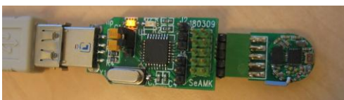
Figure 4: USB-SPI bridge with wireless node [6]
