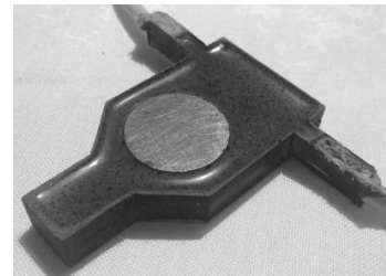
Figure 5: Resin-encapsulated 80mmX30mm temperature sensor module
