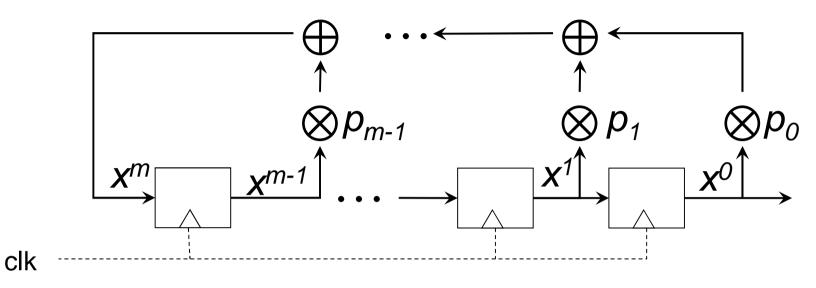
PRNGs created by LFSRs, based on Gallois field theory Feedback parameter p<sub>i</sub> determined by Primitive polynomial (Gallois Field Theory)
