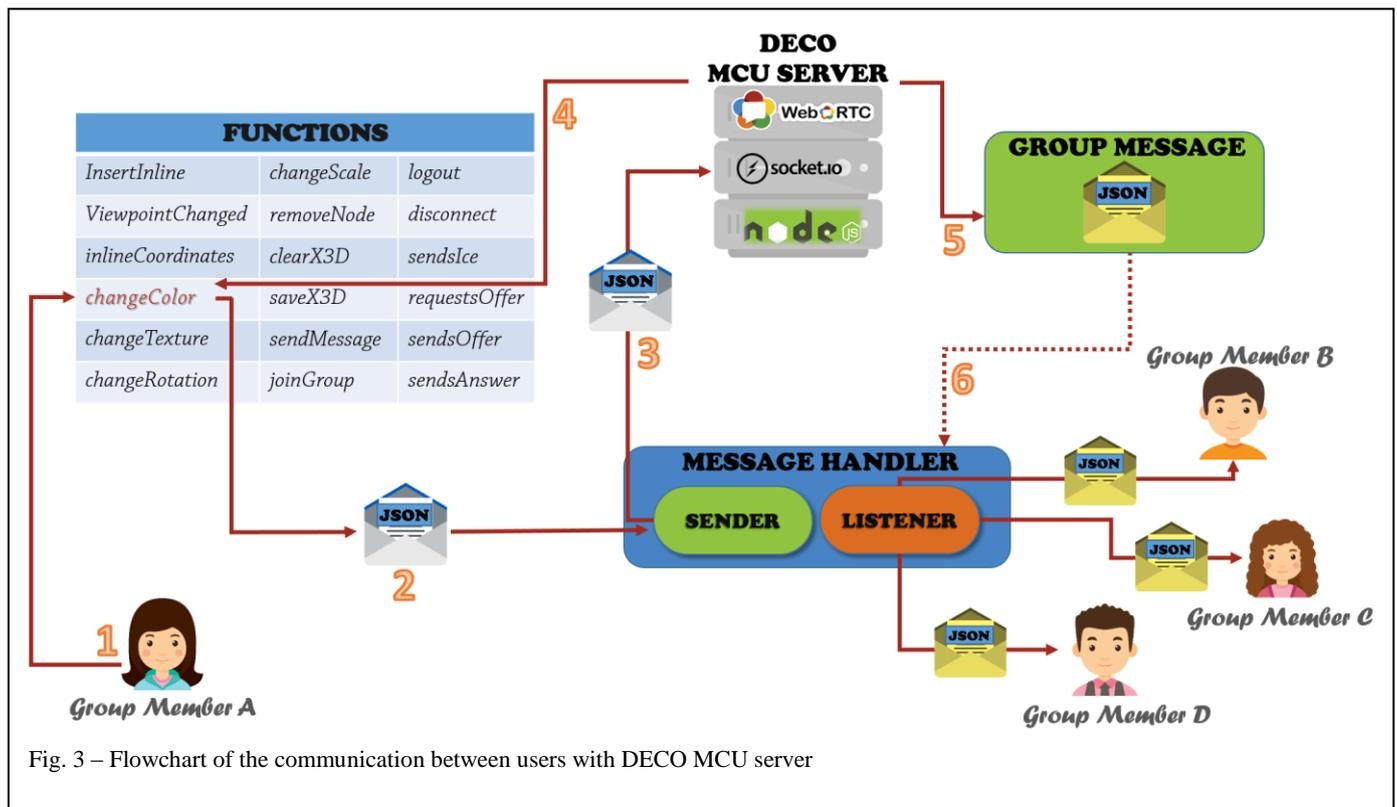
Fig. 3 – Flowchart of the communication between users with DECO MCU server
