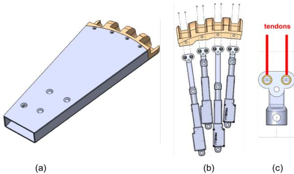
Fig. 5. (a) The CAD models of the palm, (b) the actuators of the fingers and (c) the T-shape link of the tendons.
