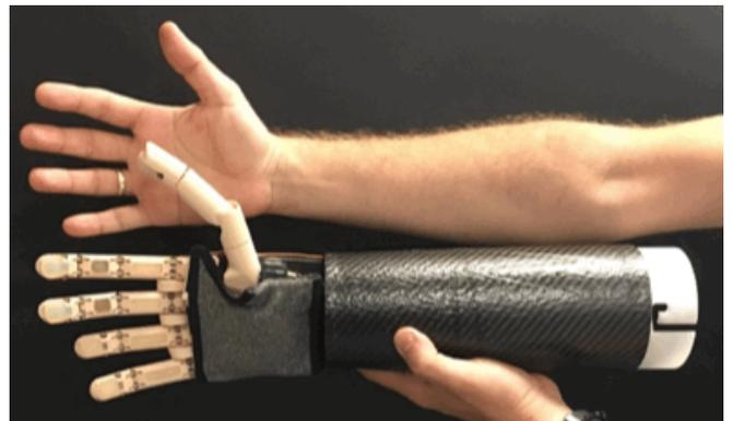
Fig. 1. The developed transradial prosthesis
