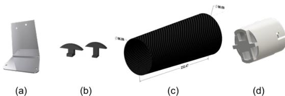
Fig. 6. The CAD models of the parts comprising the forearm: (a) the internal support plate, (b) the two wedges, (c) the external carbon fiber case and (d) the internal base as connected to the prosthetic hand.
