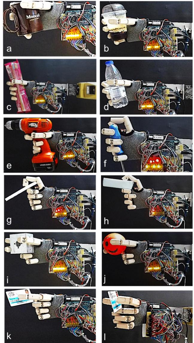
Fig. 9. The prosthetic hand grasping a variety of objects.
