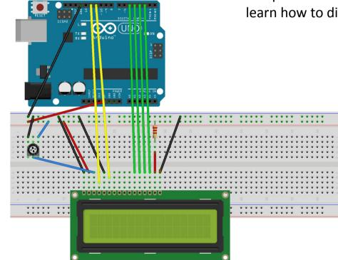
The LiquidCrystal library allows you to control LCD displays that are compatible with the Hitachi HD44780 driver. Using a LCD, students will learn how to display information.
