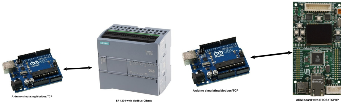
Figure 1. Example associations - Left: Arduino and S7-1200. Right: Arduino and ARM platform.
