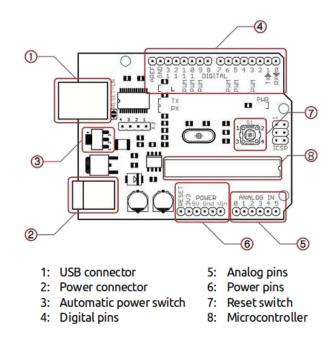
Fig. 1. Arduino Uno diagram. Source: Adapted from [6]
