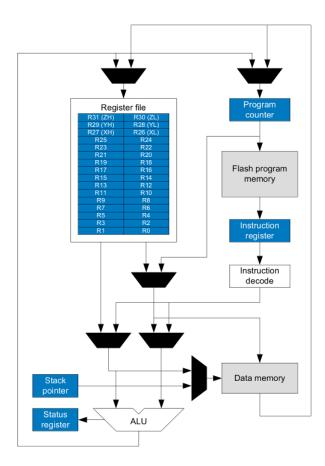
Fig. 2. AVR architecture block diagram. Source [8]
