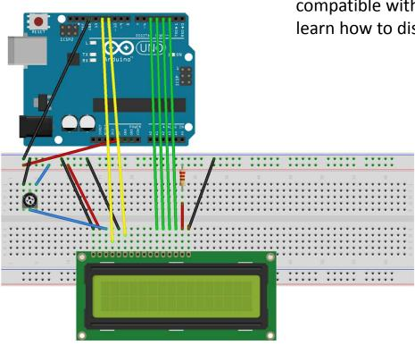
The LiquidCrystal library allows you to control LCD displays that are compatible with the Hitachi HD44780 driver. Using a LCD, students will learn how to display information.
