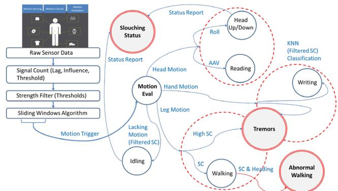
Figure 1: IC-SAFE Algorithm
