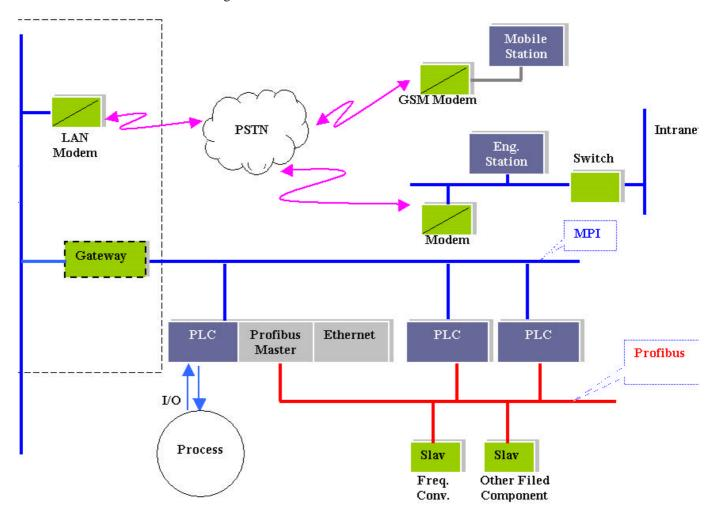
Figure 5. The modem based solution
