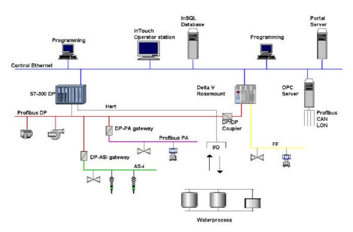
Figure 4. The system structure used in the Case Study
