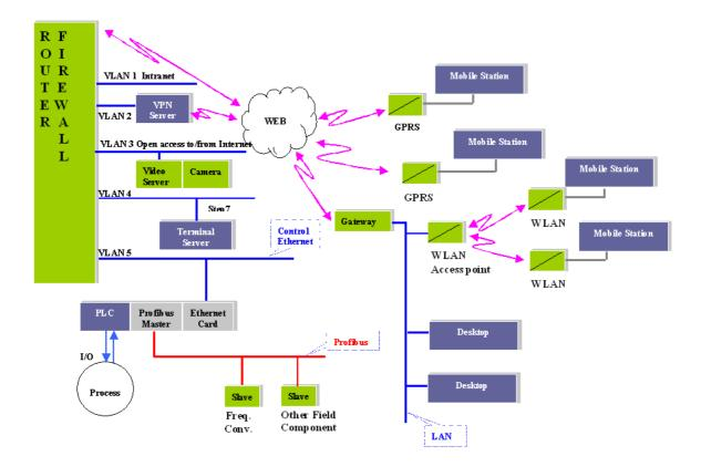
Figure 6: The Complete Network structure of the system
