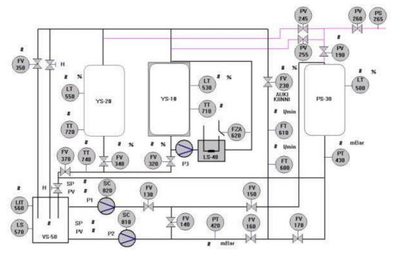
Figure 2: The PI diagram of the waterprocess
